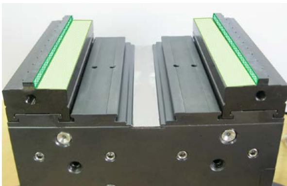
Permissible **contact surface** and **clamping surface** for the workpiece.
