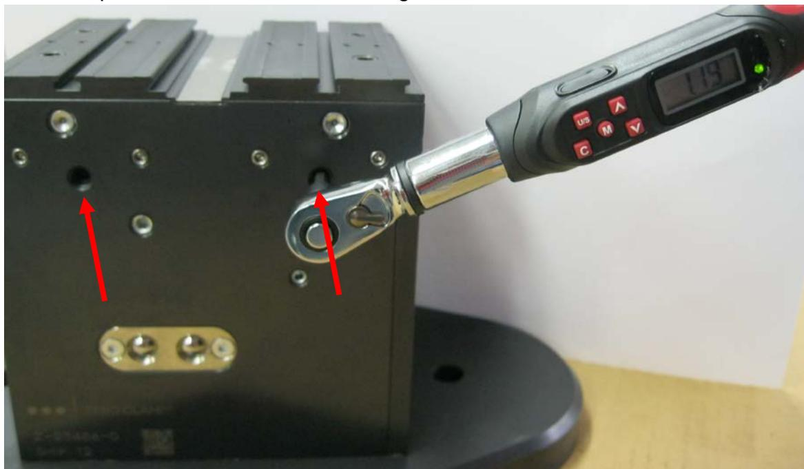
Maximum tightening torque: 1 – 2 Nm. One rotation corresponds to a center shift of  $\approx 0,33$  mm. If the center is to be shifted, remove the screw in the opposite position and pull out the pin behind the screw, e.g., with a pin puller M4. If only an excessive play is to be reduced, it is enough to retighten the screws accordingly. For this purpose, it is recommended to open the clamping vise as far as it will go.
