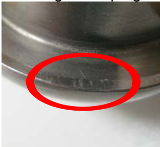
Signs of wear on a clamping stud
