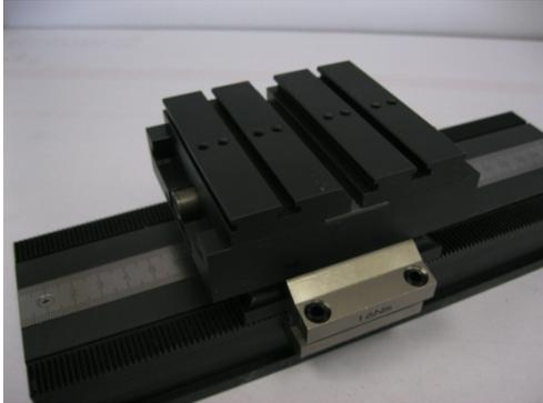
Jaw alignment in delivery state
